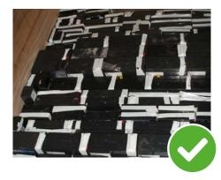
Batteries should be stored in a cool, dry **weatherproof** and supervised location. Please **close all lids**.
