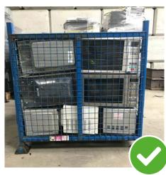
Microwaves can be placed in large WEEE cages and **stacked heaviest at the bottom, lightest at the top.**
