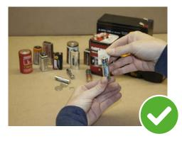
The taping of terminals is best practice and prevents the possibility of short circuit.
