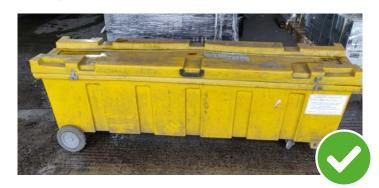
Only the **correct**receptacles may be used as pictured above and must **not be overfilled** to prevent breakage.
