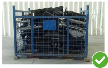
Please do not mix CRT units and FPD units in the same cage. Always load heaviest to lightest to prevent damage.
