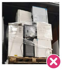
Shrink wrap to the **base** of the pallet to prevent movement in transit and **don't** overload the pallet.
