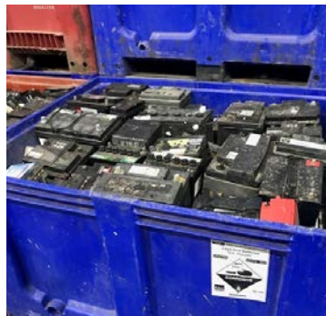
Pallet boxes containing Lead Acid batteries
